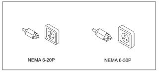
Figure 3. Plug Configurations
